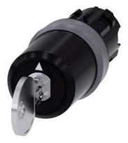
Key-operated switch BKS, 22 mm, round, plastic with metal front ring, lock number S1, with 2 keys, 3 switch positions I>O<II, momentary contact type, actuating angle 2x45°, 10:30h/12h/13:30h, key removal O, with laser labeling, inscription or symbol Customer-specific selection with SIRIUS ACT configurator (CIN)
