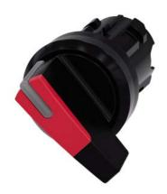
Selector switch, illuminable, 22 mm, round, plastic, red, selector switch, long, 2 switch positions O-I, latching, actuating angle  $90^\circ$ , 10:30h/13:30h, with laser labeling, upper case and lower case, always upper case at beginning of line
