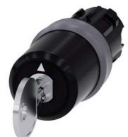
key-operated switch Siemens, 22 mm, round, plastic with metal front ring, lock number SSG10, with 2 keys, 3 switch positions I>O<II, momentary contact on the left, latching on the right, actuating angle 2x45°, 10:30h/12h/13:30h, key removal O+II, with laser labeling, inscription or symbol customer-specific selection with SIRIUS ACT configurator (CIN)
