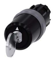
key-operated switch Siemens, 22 mm, round, plastic with metal front ring, lock number SSG10, with 2 keys, 3 switch positions I-O-II, latching, actuating angle  $2x45^\circ, 10:30h/12h/13:30h,$  key removal I+II, with laser labeling, upper case and lower case, always upper case at beginning of line
