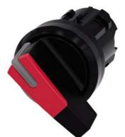
Selector switch, illuminable, 22 mm, round, plastic, red, selector switch, long, 2 switch positions O-I, latching, actuating angle 90°, 10:30h/13:30h, with laser labeling, upper case and lower case, always upper case at the beginning of the word
