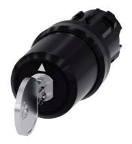
Key-operated switch BKS, 22 mm, round, plastic, lock number S1, with 2 keys, 3 switch positions I-O-II, latching, actuating angle 2x45°, 10:30h/12h/13:30h, Key removal I+II, with laser labeling, upper case and lower case, always upper case at beginning of line
