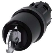
Key-operated switch IKON, 22 mm, round, plastic, lock number 360012K1, with 2 keys, 3 switch positions I-O-II, latching, actuating angle 2x45°, 10:30h/12h/13:30h, key removal O, with laser labeling, upper case and lower case, always upper case at beginning of line
