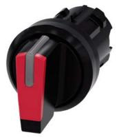
Selector switch, illuminable, 22 mm, round, plastic, red, selector switch, short, 3 switch positions I>O<II, momentary contact type, actuating angle  $2x45^{\circ}$ , 10:30h/12h/13:30h, with laser labeling, lower case
