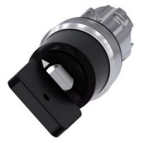
key-operated switch Siemens, 22 mm, round, metal, shiny, lock no. VL5, with 2 keys, 2 switch positions O-I, latching, actuating angle  $90^\circ$ , 10:30h/13:30h, key removal O, with laser labeling, upper case
