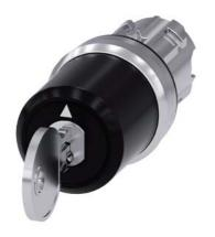
Key-operated switch BKS, 22 mm, round, metal, shiny, special lock, with 2 keys, 3 switch positions I-O-II, latching, actuating angle 2x45°, 10:30h/12h/13:30h, key removal I, Note: BKS locking systems E1 - E25 supplied without key
