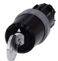
Key-operated switch BKS, 22 mm, round, plastic with metal front ring, special lock, with 2 keys, 3 switch positions I-O-II, latching, actuating angle 2x45°, 10:30h/12h/13:30h, key removal I+O+II, Note: BKS locking systems E1 - E25 supplied without key
