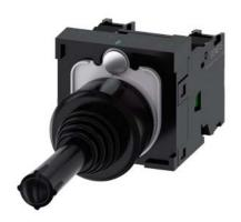
Coordinate switch, 22 mm, round, plastic, black, 2 switch positions, horizontal latching, without mechanical interlocking, in O position, with holder, 1 NO, 1 NO, screw terminal, with laser labeling, upper case and lower case, always upper case at the beginning of the word
