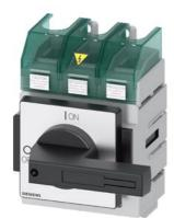
SENTRON, Molded case switch 3LD5 UL, Main switch, 3-pole, certified according to UL489 UL60947-4-1 and IEC60947-3, UL: 150A, SCCR 50kA at 480VAC, Operating power at 480VAC 3-phase: 100hp, IEC: 160A, Operating power at AC-23A at 400V: 75kW, floor mounting with direct handle, black, incl. terminal covers for the infeed side
