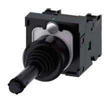
Coordinate switch, 22 mm, round, plastic, black, 2 switch positions, horizontal, momentary contact type, with mechanical interlocking in O position, with holder, 1 NO, 1 NO, screw terminal, with laser labeling, upper case and lower case, always upper case at the beginning of the word
