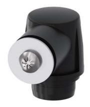
Twist lever operating mechanism Functional at -40 °C For position switch 3SE51 For 40/56/56XL mm, Switching points according to EN 50041. The switching direction of the levers can be set to left/right or only left or only right. Delivery condition is left/right. (Please order lever separately)
