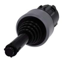
Coordinate switch, 22 mm, round, plastic with metal front ring, black, 4 switch positions, momentary contact type, with mechanical interlocking, with laser labeling, upper case
