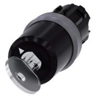
key-operated switch Siemens, 22 mm, round, plastic with metal front ring, lock no. LSG1, with 2 keys, 2 switch positions O-I, latching, actuating angle  $90^\circ, 10:30h/13:30h,$  key removal O, Z=50-unit packaging
