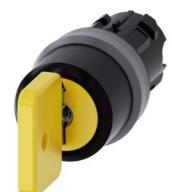
Key-operated switch O.M.R, 22 mm, round, plastic with metal front ring, lock number 73033, yellow, with 2 keys, 3 switch positions I-O-II, latching, actuating angle 2x45°, 10:30h/12h/13:30h, Key removal I+O+II, with laser labeling, upper case and lower case, always upper case at the beginning of the word
