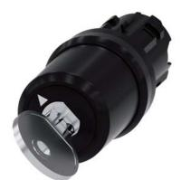
Key-operated switch BKS, 22 mm, round, plastic, Lock No. E7 (VW), without key, 2 switch positions O-I, latching, actuating angle 90°, 10:30h/13:30h, key removal O+I, with laser labeling, upper case and lower case, always upper case at beginning of line
