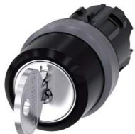
RONIS key-operated switch, 22 mm, round, plastic with metal front ring, special lock, with 2 keys, 3 switch positions I-O<II, left latching, right momentary contact type, actuating angle  $2x45^{\circ}$ , 10:30h/12h/13:30h, key removal O, possible special locks: SB31, 421, 455
