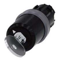
Key-operated switch BKS, 22 mm, round, plastic with metal front ring, lock number S1, with 2 keys, 2 switch positions O-I, latching, actuating angle  $90^{\circ}$ , 10:30h/13:30h, key removal O+I, with laser labeling, upper case
