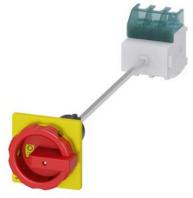
SENTRON, Switch disconnector 3LD, emergency switching-off switch, 3- pole, lu: 63 A, operating power / at AC-23 A 400 V: 22 kW, floor mounting with door coupling, rotary operating mechanism, Red / yellow, central mounting 22.5 mm of the handle
