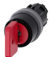
Key-operated switch O.M.R, 22 mm, round, plastic with metal front ring, lock number 73037, red, with 2 keys, 3 switch positions I-O-II, latching, actuating angle 2x45°, 10:30h/12h/13:30h, key removal O+I, with laser labeling, inscription or symbol Customer-specific selection with SIRIUS ACT configurator (CIN)
