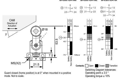
Maximum allowable travel varies by model and is listed at bottom of switching diagram (minus operating tolerance). Switching Angles ( $\theta$ ) are measured with actuating system in vertical position (as drawn) and are applicable both left and right movement.
