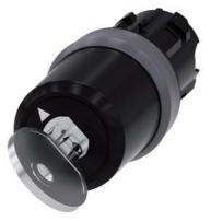
Key-operated switch BKS, 22 mm, round, plastic with metal front ring, Lock number E1 (VW), without key, 2 switch positions O-I, latching, actuating angle  $90^{\circ}$ , 10:30h/13:30h, key removal O+I, with laser labeling, upper case and lower case, always upper case at the beginning of the word
