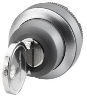
key-operated switch for extension units, 22mm, round, plastic, latching, 3 switch positions 1-0-2, 2 NO contacts, with 2 keys (incl. printed-circuit board, contact module)
