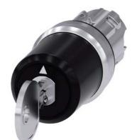
key-operated switch Siemens, 22 mm, round, metal, shiny, lock no. STGH10, with 2 keys, 3 switch positions I-O<II, left latching, momentary contact type on the right, actuating angle 2x45°, 10:30h/12h/13:30h, key removal O+I, with laser labeling, upper case
