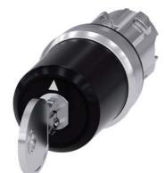
Key-operated switch BKS, 22 mm, round, metal, shiny, special lock, with 2 keys, 3 switch positions I-O<II, latching on the left, momentary contact type on the right, actuating angle 2x45°, 10:30h/12h/13:30h, key removal O, Note: BKS locking systems E1 - E25 supplied without key
