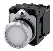
Illuminated pushbutton, 22 mm, round, metal, shiny, white, pushbutton, flat, momentary contact type, with holder, 1 NO, LED module with integrated LED 24 V AC/DC screw terminal
