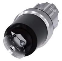
Key-operated switch IKON, 22 mm, round, metal, shiny, lock number 360012K1, with 2 keys, 2 switch positions O-l, latching, actuating angle  $90^\circ$ , 10:30h/13:30h, key removal O+l, Z=50-unit packaging
