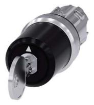
Key-operated switch BKS, 22 mm, round, metal, shiny, lock number S1, with 2 keys, 3 switch positions I-O-II, latching, actuating angle 2x45°, 10:30h/12h/13:30h, Key removal I+O+II, with laser labeling, upper case and lower case, always upper case at the beginning of the word
