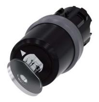
Key-operated switch BKS, 22 mm, round, plastic with metal front ring, lock number S1, with 2 keys, 2 switch positions O-I, latching, actuating angle  $90^\circ, 10:30h/13:30h,$  key removal O, with laser labeling, upper case and lower case, always upper case at beginning of line
