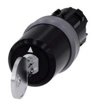
Key-operated switch BKS, 22 mm, round, plastic with metal front ring, lock number S1, with 2 keys, 3 switch positions I>O<II, momentary contact type, actuating angle  $2x45^{\circ}$ , 10:30h/12h/13:30h, key removal O, with laser labeling, upper case and lower case, always upper case at beginning of line
