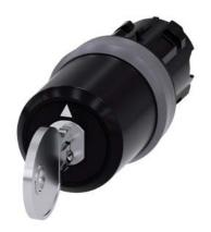
Key-operated switch BKS, 22 mm, round, plastic with metal front ring, lock number S1, with 2 keys, 3 switch positions I-O-II, latching, actuating angle 2x45°, 10:30h/12h/13:30h, key removal I, with laser labeling, upper case and lower case, always upper case at the beginning of the word
