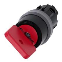
Key-operated switch O.M.R, 22 mm, round, plastic with metal front ring, lock number 73037, red, with 2 keys, 2 switch positions O-I, latching, actuating angle 90°, 10:30h/13:30h, Key removal O+I
