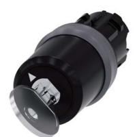
Key-operated switch BKS, 22 mm, round, plastic with metal front ring, Lock No. E2 (VW), without key, 2 switch positions O-I, latching, actuating angle 90°, 10:30h/13:30h, key removal O+I, with laser labeling, upper case and lower case, always upper case at the beginning of the word
