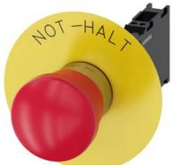
EMERGENCY STOP mushroom-type actuator, 22 mm, round, metal, shiny, red, 40 mm, positive latching, according to EN ISO 13850, pull-to-unlatch mechanism, with yellow backing plate, inscription: NOT-HALT, with holder, 1 NO+1 NC, spring-type terminal, Z=20-unit packaging
