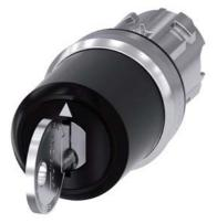
Key-operated switch IKON, 22 mm, round, metal, shiny, lock number 360012K1, with 2 keys, 3 switch positions I>O<II, momentary contact type, actuating angle 2x45°, 10:30h/12h/13:30h, key removal O, Z=50-unit packaging
