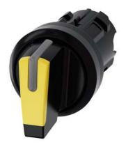
Selector switch, illuminable, 22 mm, round, plastic, yellow, selector switch, short, 3 switch positions I-O<II, left latching, right momentary contact type, actuating angle 2x45°, 10:30h/12h/13:30h, with laser labeling, inscription or symbol Customer-specific selection with SIRIUS ACT configurator (CIN)
