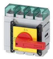
SENTRON, Molded case switch 3LD5 UL, Emergency switching-off, 4-pole, certified according to UL489 UL60947-4-1 and IEC60947-3, UL: 125A, SCCR 65kA at 480VAC, Operating power at 480VAC 3-phase: 75hp, IEC: 125A, Operating power at AC-23A at 400V: 55kW, front-mounted, rotary operating mechanism, red/yellow, 4-hole mounting of the handle, incl. terminal covers for the infeed side
