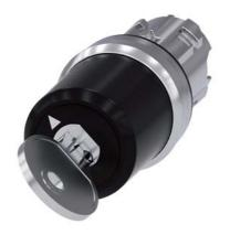
Key-operated switch BKS, 22 mm, round, metal, shiny, Lock No. E7 (VW), without key, 2 switch positions O-l, latching, actuating angle  $90^\circ$ , 10:30h/13:30h, key removal O+l, with laser labeling, upper case and lower case, always upper case at the beginning of the word
