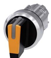
Selector switch, illuminable, 22 mm, round, metal, shiny, amber, selector switch, short, 3 switch positions I>O<II, momentary contact type, actuating angle  $2x45^{\circ}$ , 10:30h/12h/13:30h
