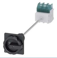
SENTRON, Switch disconnector 3LD, main switch, 3-pole, lu: 63 A, Operating power / at AC-23 A at 400 V: 22 kW, floor mounting with door coupling, rotary operating mechanism, black, central mounting 22.5 mm of the handle
