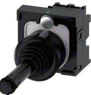
Coordinate switch, 22 mm, round, plastic, black, 2 switch positions, vertical latching, with mechanical interlocking, in O position, with holder, 1 NO, 1 NO, screw terminal, Z=20-unit packaging
