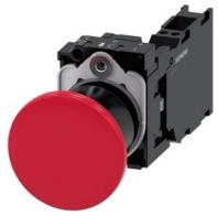
Mushroom pushbutton, 22 mm, round, plastic, red, 40mm, latching, pull-to-unlatch mechanism, with holder, 1 NO+1 NC, spring-type terminal, with laser labeling, upper case and lower case, always upper case at the beginning of the word
