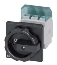
SENTRON, Switch disconnector 3LD, main switch, 3-pole, lu: 25 A, Operating power / at AC-23 A at 400 V: 9.5 kW, front-mounted, rotary operating mechanism, black, central mounting 22.5 mm of the handle
