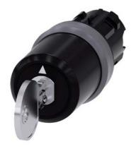
Key-operated switch BKS, 22 mm, round, plastic with metal front ring, lock number S1, with 2 keys, 3 switch positions I>O<II, momentary contact on the left, latching on the right, actuating angle  $2x45^{\circ}$ , 10:30h/12h/13:30h, key removal O, with laser labeling, upper case
