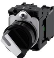
Selector switch, illuminable, 22 mm, round, plastic, white, selector switch, short, 2 switch positions O-I, latching, 10:30h/13:30h, with holder, 1 NO, 1 NC, screw terminal, Z=20-unit packaging
