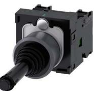
Coordinate switch, 22 mm, round, plastic with metal front ring, black, 2 switch positions, horizontal latching, with mechanical interlocking, in O position, with holder, 1 NO, 1 NO, screw terminal,
