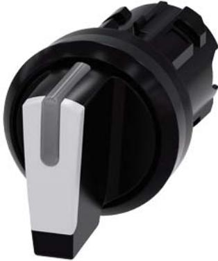
Selector switch, illuminable, 22 mm, round, plastic, white, selector switch, short, 3 switch positions I>O<II, momentary contact on the left, latching on the right, actuating angle 2x45°, 10:30h/12h/13:30h, with laser labeling, upper case and lower case, always upper case at the beginning of the word
